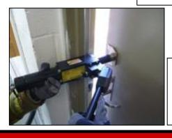
3. **Spread**. Begin with small pumps to maintain your bite. Use the axe or a wedge to capture your progress and be prepared to control the door. Reposition and repeat if necessary.
