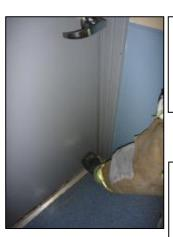
1. **Gap** the door. Shock the door as you would normally to size up the door and identify additional locks. Push your foot on the bottom of the door to create a gap for the Hydra-Ram. Use a Halligan if necessary.
