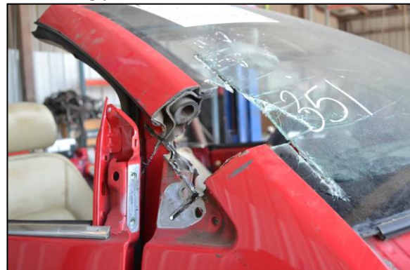
Boron steel pipe in the "A" post of a VW Beetle
