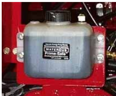
Figure 4-2: Primer Pump Lubrication Fluid or Oil Reservoir
