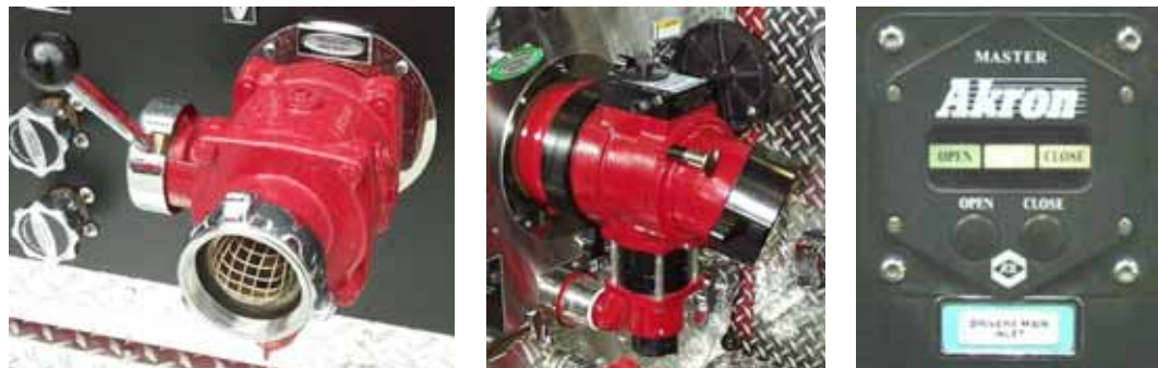
Figure 3-4: Typical Gated Intake Valves
