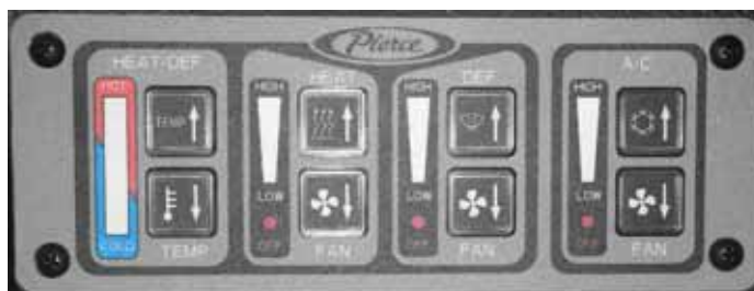
Figure 4-5: HVAC Control Panel
