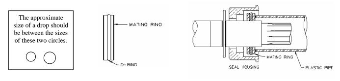
4. Clean the mating ring surface with isopropyl alcohol to remove any fingerprints and any other contaminants left on mating ring.
