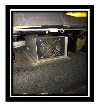
Engine/ Truck- Be cautious on placement of equipment inside compartments with 120 v outlet covers. As the covers are being broken off by unsecured equipment.
