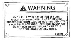
5. The weight of personnel and equipment suspended from the ladder must be deducted from the tip load allowance as shown on the aerial load chart.
